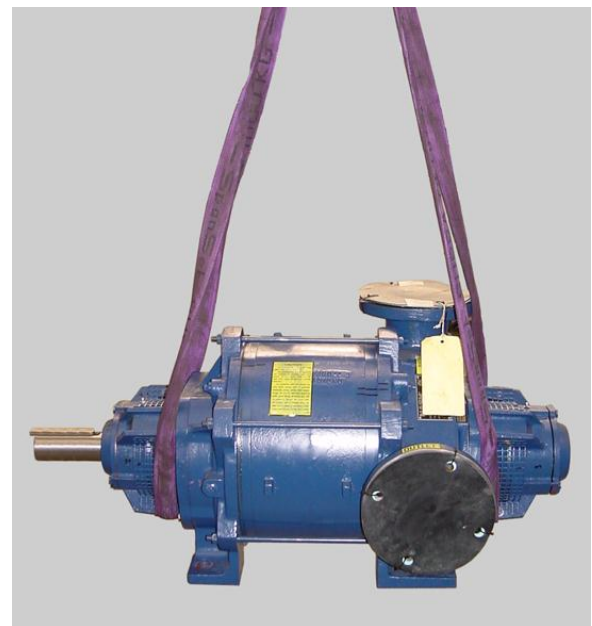
Fig. 4 Fastening lifting gear to individual machines
